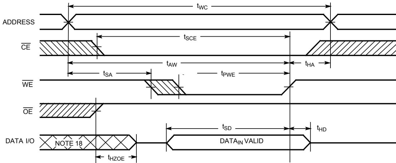
**Write Cycle No. 3 ( $\overline{WE}$  Controlled,  $\overline{OE}$  LOW)<sup>[17]</sup>**
